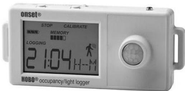
Fig. 2. The HOBO UX90-005M Room Occupancy/Light Logger that was used during the study.
